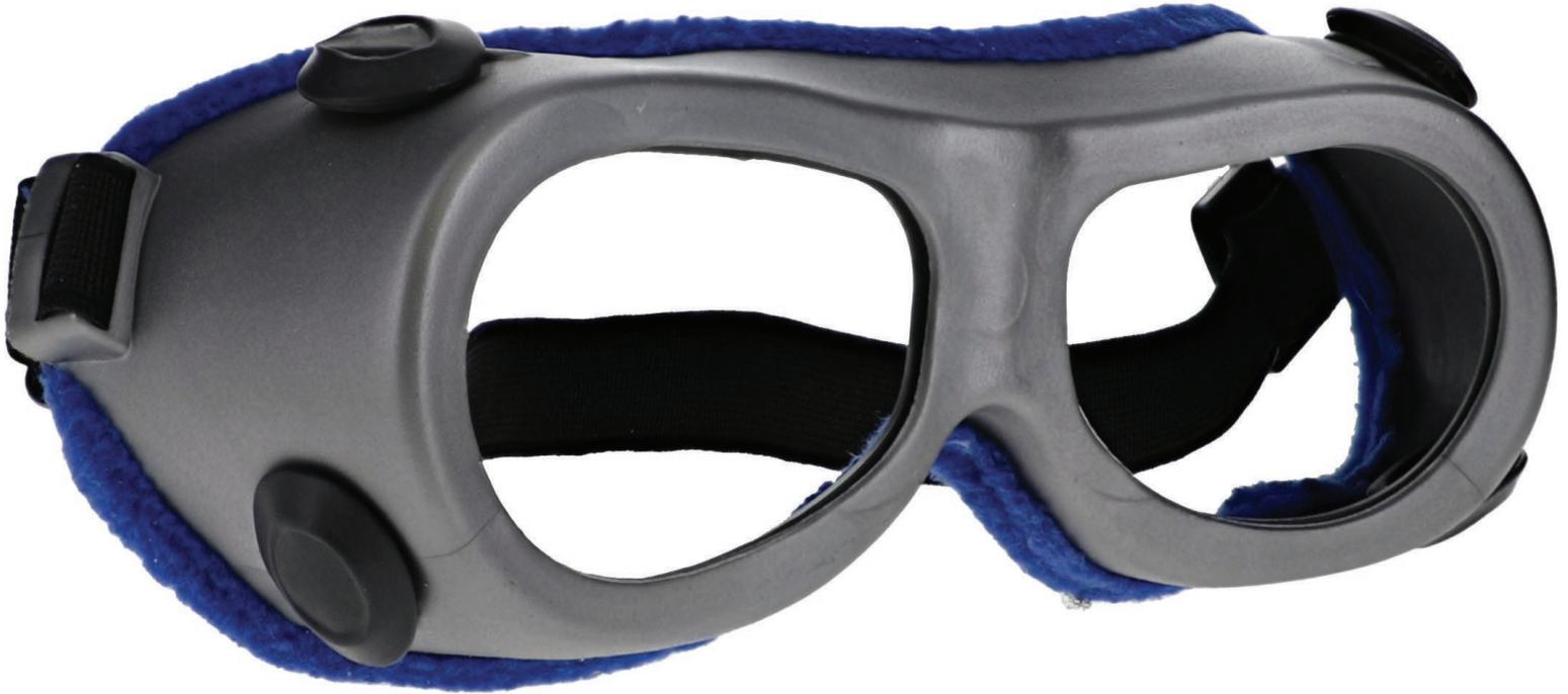
The CR39 laser safety glasses have a polycarbonate clear lens filter that provides laser protection. These laser glasses have visible light transmission of 85%. In addition, the CR39 laser safety glasses have ANSI Z87.1 and ANSI Z136.1 safety standards, and CE certified lens. These laser safety goggles 55 is a durable and lightweight fitover goggles frame. Made of high-quality plastic, the 55 laser safety goggles feature strap. These Phillips Safety laser safety goggles are available in silver.
