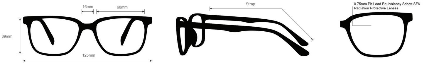
The radiation glasses RK2 feature high quality, distortion-free SF-6 Schott glass radiation-reducing lenses with 0.75mm Pb lead equivalency protection. The RK2 lead glasses have clear CE Certified Lens and weight 85 g. These radiation goggles RK2 are prescription available. Made of high-quality plastic, it is a durable and lightweight goggles frame. The RK2 radiation goggles feature foam eyecup and strap. These Phillips Safety prescription radiation goggles are available in black.
