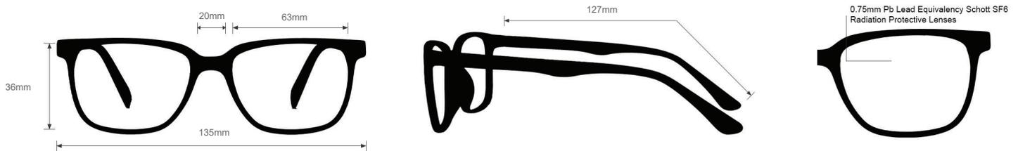
The radiation glasses P820 feature high quality, distortion-free SF-6 Schott glass radiation-reducing lenses with 0.75mm Pb lead equivalency protection. The P820 lead glasses have clear CE Certified Lens and weight 78g. These radiation glasses P820 are non-prescription. Made of high-quality plastic, it is a durable and lightweight wrap around frame. The P820 radiation glasses feature rubberized nose pads. These Phillips Safety radiation glasses are available in black and silver.
