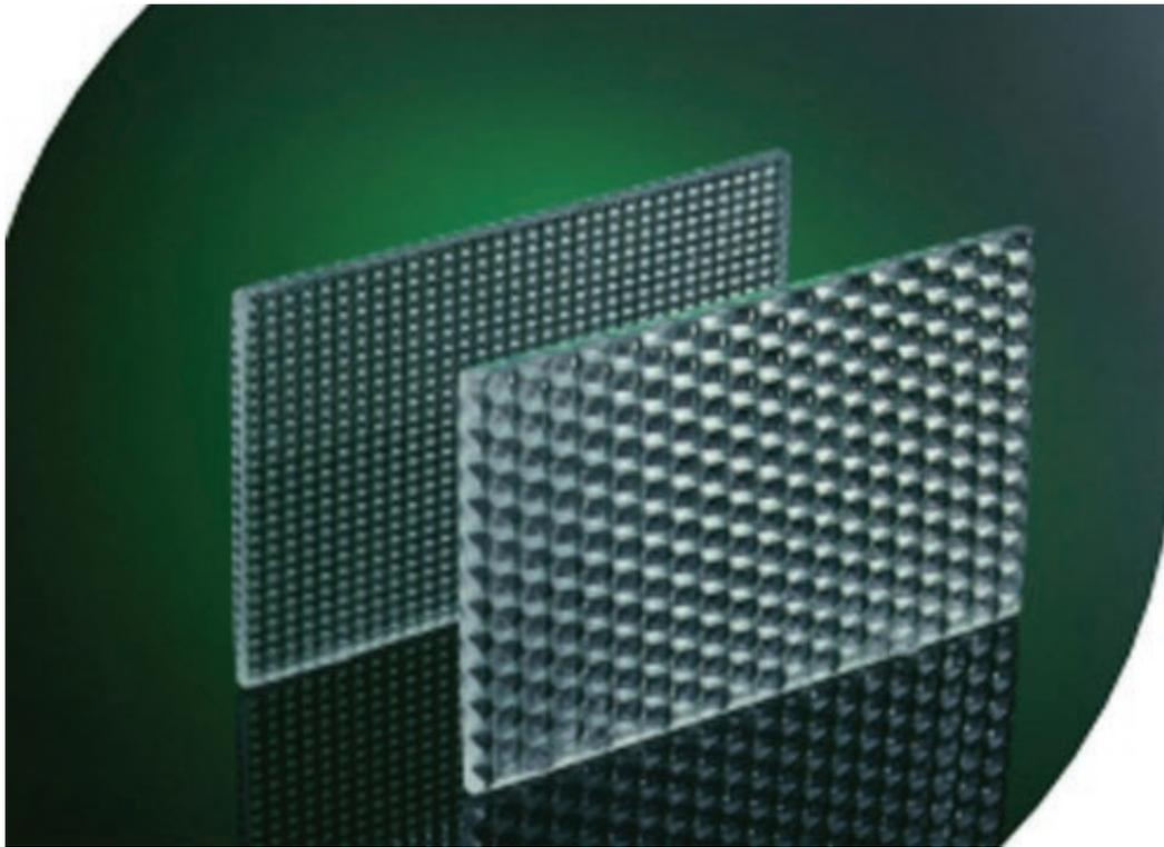
Pattern glass creates visual interest and varying levels of opacity by creating a subtle shifting of light, which makes pattern glass the ideal choice for a wide range of applications. The process of fabricating pattern glass involves pressing semi-molten glass between metal rollers or with a single roller and a calendering table to provide a distinct look.
