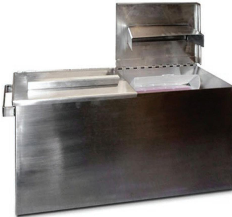
The Shielded Sharps Container provides a simple, safe and convenient solution for the disposal of used syringes that may be contaminated with high-energy radionuclides. It features convenient lifting handles and has a key-lockable, hinged top. With 0.5 and 1.0 inch lead shielding, it accommodates any size sharps container. As with all of our products, Phillips Safety can design and manufacture a custom shielded sharps container to meet your exact specifications.
