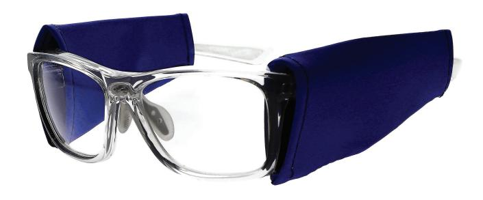
The Universal Radiation Protective Side Shields by Phillips Safety are an innovative lateral eye radiation protection. They are made with our nylon covered leaded vinyl and provide optimum hygiene properties. These leaded side shields can be easily added to any eyewear and replaced when necessary. They have a Lead Equivalency of 0.25mm Pb. In addition, the Universal Radiation Protective Side Shields are available in 3 colors: black, purple, and blue.
